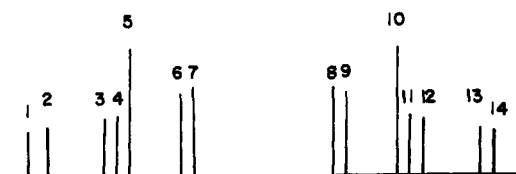
Figure 2. Schematic slow-exchange spectrum of SF 4 .
